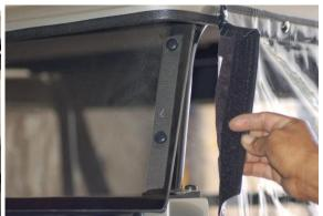
10) Drill holes for other snaps after corner snaps and velcro have been applied.
