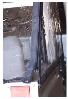
Put on other door section in same manner. Zip to rear section. Pull to add tension, then apply corner snaps first.
