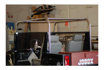
2) Insert 2x4" (shown) bolts in the 4 corner holes and 2 frame leg holes.
