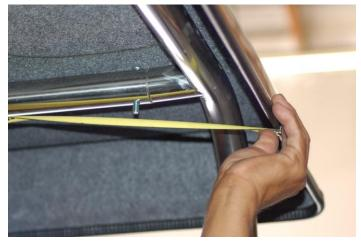
Use curtain to make sure hardtop is aligned adequately on both sides. Line curtain along the ridge of the roof lip.
