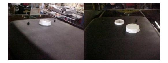
2. Check water level gauge and fill unit with WATER only. **DO NOT** fill unit past red marker on gauge.
